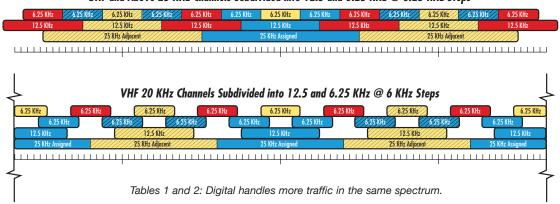
UHF and Above 25 KHz Channels Subdivided into 12.5 and 6.25 KHz @ 6.25 KHz Steps
