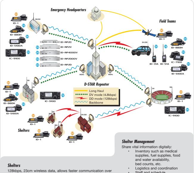
areas of several miles\* for Ethernet-based communications while offering secure receive and transmit information.
