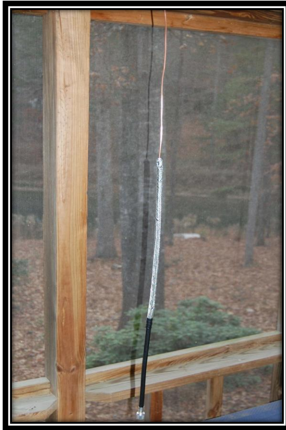
Figure 4. Example of VHF Coaxial Sleeve Antenna
