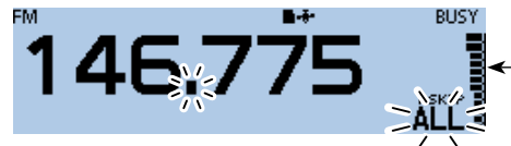
The S-meter displays the received signal strength.
