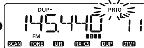
Pauses on a memory or call channel when a signal is received.
